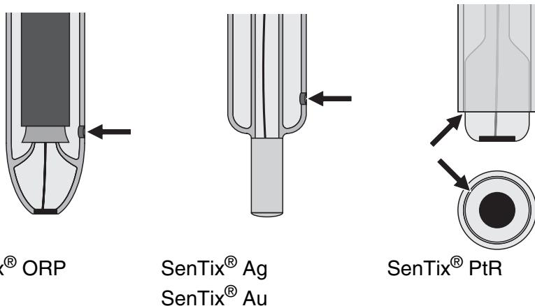
SenTix® ORPIL, SenTix® Au and SenTix® Ag: The level of the reference electrolyte must be at least 2 cm above the level of the solution.
